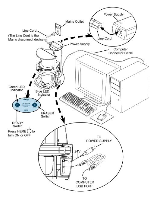
Figure 1. Typical ScanX Installation
